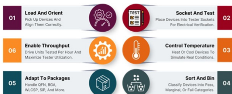
Figure 1: Core functions of a semiconductor test handler
