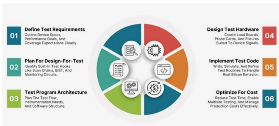
Figure 1: Key steps in developing ATE test programs
