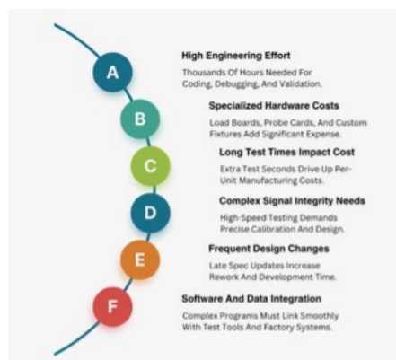
Figure 2: The cost and complexity of ATE test programs
