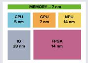
Disaggregated fabrication with blocks using different technology nodes
