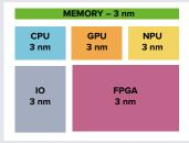
Aggregated fabrication with all the blocks using one specific technology node
