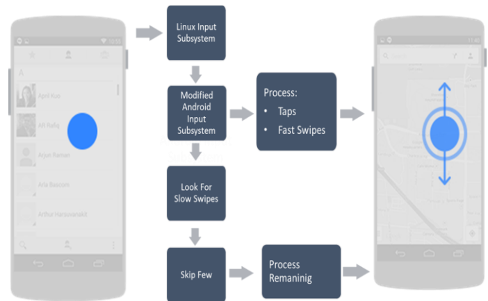
FIGURE 13: INTERRUPT SKIPPING MODEL OF TOUCH PROCESSING
